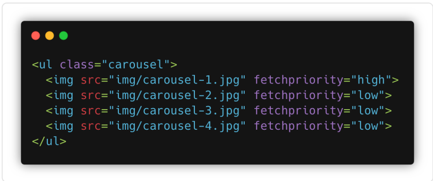
Figure 18.21. Fetch Priority API example to improve image loading behaviour in a carousel component.
